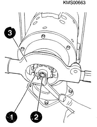
CHECKING RETURN FORCE OF COIL SPRING ON ENGAGEMENT ROD
